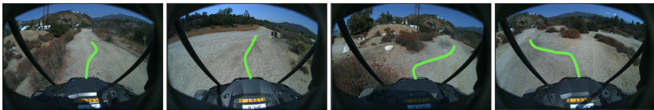
Fig. 6: Example observations from our evaluations, with the vehicle’s future path visualized in green. Our system can learn from the training data and expert corrective behavior to learn autonomous trail-following behavior directly from egocentric visual observations.
