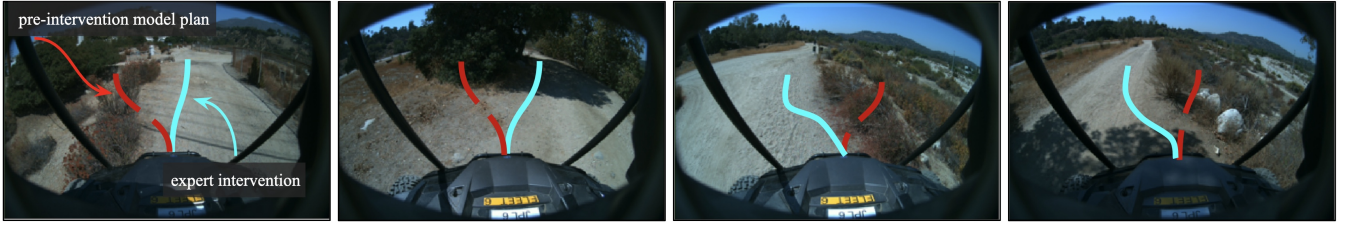
Fig. 4: Example intervention scenes used for training. The deployed imitative policy often makes wrong predictions (plans shown in red), requiring a human expert to intervene and provide corrective behavior (shown in cyan). We use this corrective behavior as training data to continually improve our system.
