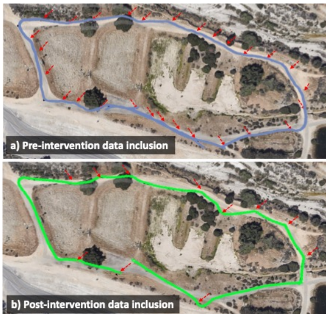
Fig. 7: Satellite view showing the human interventions made to our autonomous imitation-based system driving over the course of a dirt loop: before (top) and after (bottom) performing a round of training with the included interventions. Each arrow indicates a location at which the human intervened.
